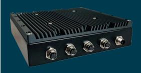
BC17 Series are fanless and extremely tough computers with IP66 rating. They are superior to industrial embedded systems and can work and endure in much more unstable environments. They have strengthened frames, M12 connections and patented technology for wide-temp operation from -25°C to 60°C.
