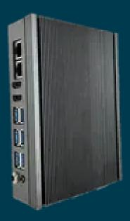
BC16 creates a more harmonized Intel 11 Gen. processors for industrial DIN rail system, industrial manufacturing needed an industrial PC (IPC) that could act as a central control system. This IPC could combine various software assets from different origins, as well as their own exclusive software.
